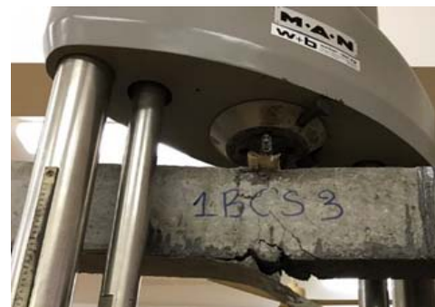
Fig.10. Rupture along direction of GFRP of strengthened beam in the mode of cover separation
