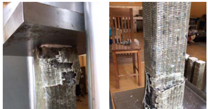
Fig.7. Failure by compression at top and bottom
